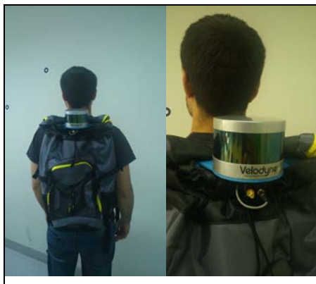
Fig. 1. Acquisition system (left), and detail of the sensors (right)
