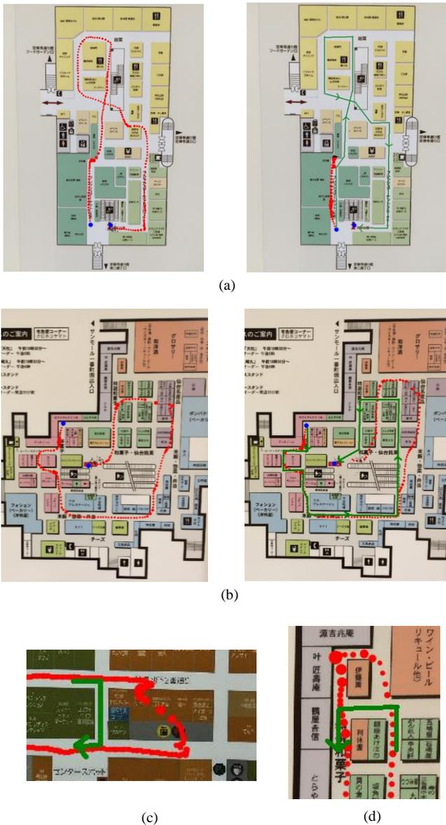
Figure 5. Result of the estimation paths: red points indicate estimated position and green lines are real paths.
